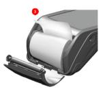
Hold the terminal securely in one hand. With the other hand, and by using two fingers, lift the printer cover release as shown in • and • above. Fully open the printer cover and remove the old roll of paper.
